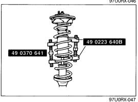
Disassembly note Coil spring and mounting plate
